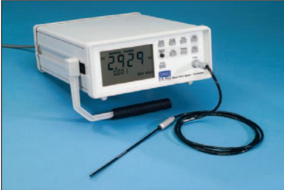
The Model 6010 Hall-effect Gauss/Tesla-Meter features F.W. Bell's exclusive Dynamic Probe Correction, along with temperature compensation and allows measurements up to 300 kG with a basic accuracy of 0.25%. Key features include Peak Hold, Max/Min Hold, Auto Zero, Auto Range, Relative Mode and Temperature measurement. The Model 6010 allows the user to select Gauss, Tesla or Ampere/Meter readings. The Model 6010 also features a corrected analog output ( $\pm 3$  V Full Scale for each range),
