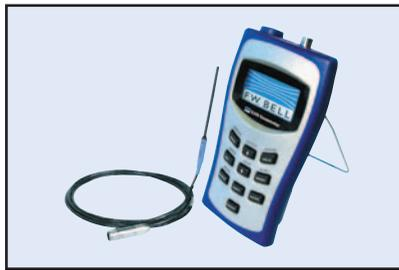
The 5100 Series Hall effect portable gaussmeters represent the most recent design from the world leader in magnetic measuring equipment. This new design incorporates the use of digital signal processing technology making it the world's first hand-held gaussmeter to have a digital signal processor (DSP) on board. F.W. Bell's exclusive Dynamic Probe Correction allows measurements from 0 to 30 kG with a basic accuracy of 1%.
